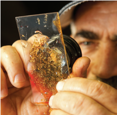
Silvio Megia checks a sample from one of LaSuCa’s vacuum pans, where sugar crystals grow in the massecuite. “Working the pans is an art,” Mike Comb says.
