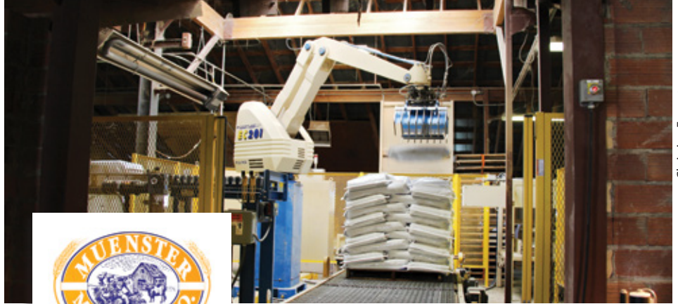
A robotic arm — part of a packaging system that was added in 2008 — grasps each bag from a conveyor and stacks it on a pallet for shipping.
